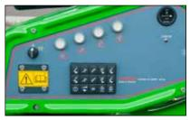
Lower controls enable the lift to be operated from ground
