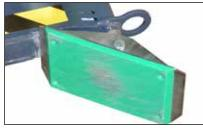
Plastic pads (4 pcs) on outrigger plates protect the surface from outrigger marks
