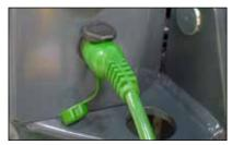
Engine heater for cold temperatures
