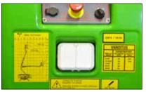
Two outlets 230 V (110 V) at platform provide electricity for power tools
